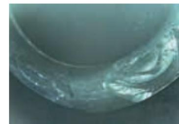
**Grease swelling** – EPDM swells in mineral oil and mineral fat and becomes softer. The damage is evident in shell-like disruptions with relatively round edges. Even individual pieces can break off. It is necessary to check whether the correct assembly grease was used. Generally, EPDM may only be lubricated with silicone grease. In addition, the product-specific information, such as fat concentration, temperature etc., should be recorded in order to verify the possibility of using EPDM.
