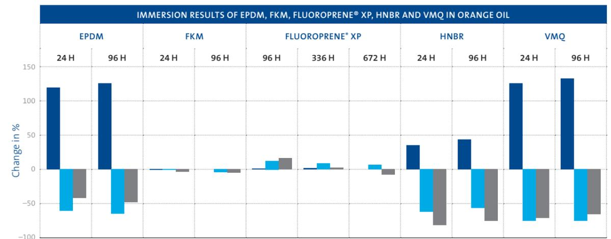
VMQ and EPDM materials clearly swell far too much in orange oil. Even the swelling behavior of HNBR exceeds the tolerable limit. Fluororubbers, on the other hand, are very resistant.
