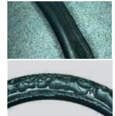
**Gap extrusion** – Provided that the design is consistent, the factors which can push the O-ring into a gap and lead to a shearing-off include varying pressures, dynamic stress and media expansion. Depending on the individual case, there are diverse manifestations, as shown in the sample illustrations above. With dynamically stressed seals, one colloquially refers to “mouse nibbling” in the event of damage.
