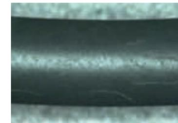
**Explosive decompression** – Cracks in longitudinal directions can be found on the surface. The elastomer saturates itself with gas under pressure. When rapid depressurization occurs, the amount of gas cannot escape fast enough from the matrix of the elastomer and forms gas bubbles (similar to diver's paralysis/aeroembolism).
